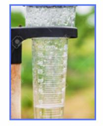
A rain gauge measures liquid precipitation across a certain range. Rain gauges vary depending on the diameter of the funnel.
