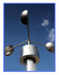
An anemometer is an instrument used to determine wind speed and direction.
