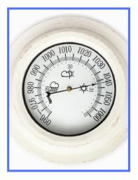
A barometer is an instrument used to measure atmospheric pressure. in order to predict the weather and determine altitude.
